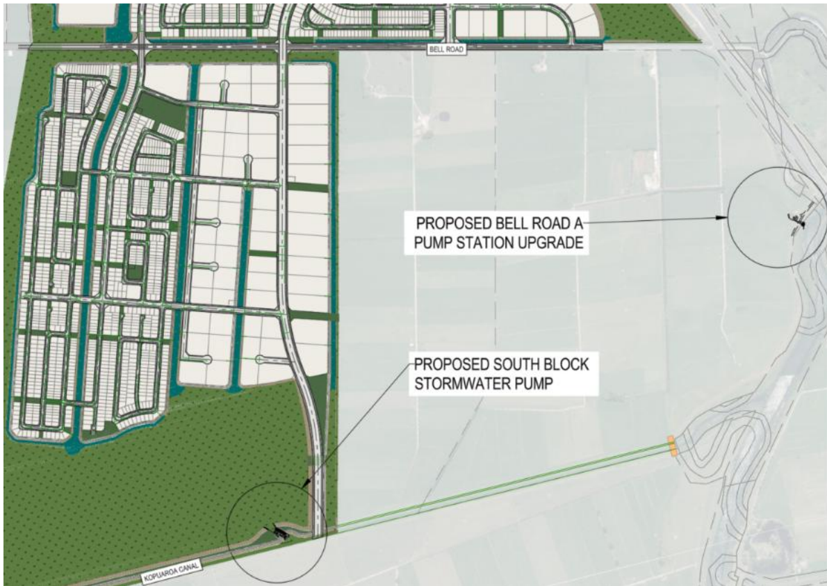
Figure 35: Stormwater Pump Locations (Source: Maven)
