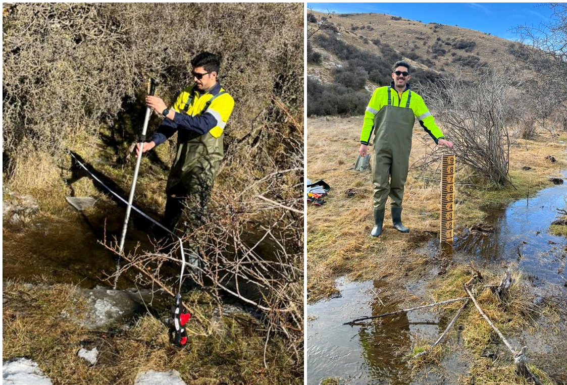
Figure 5: Flow gauging at RAS1-SW1 (left) and installed flow gauging board at same location (right).
