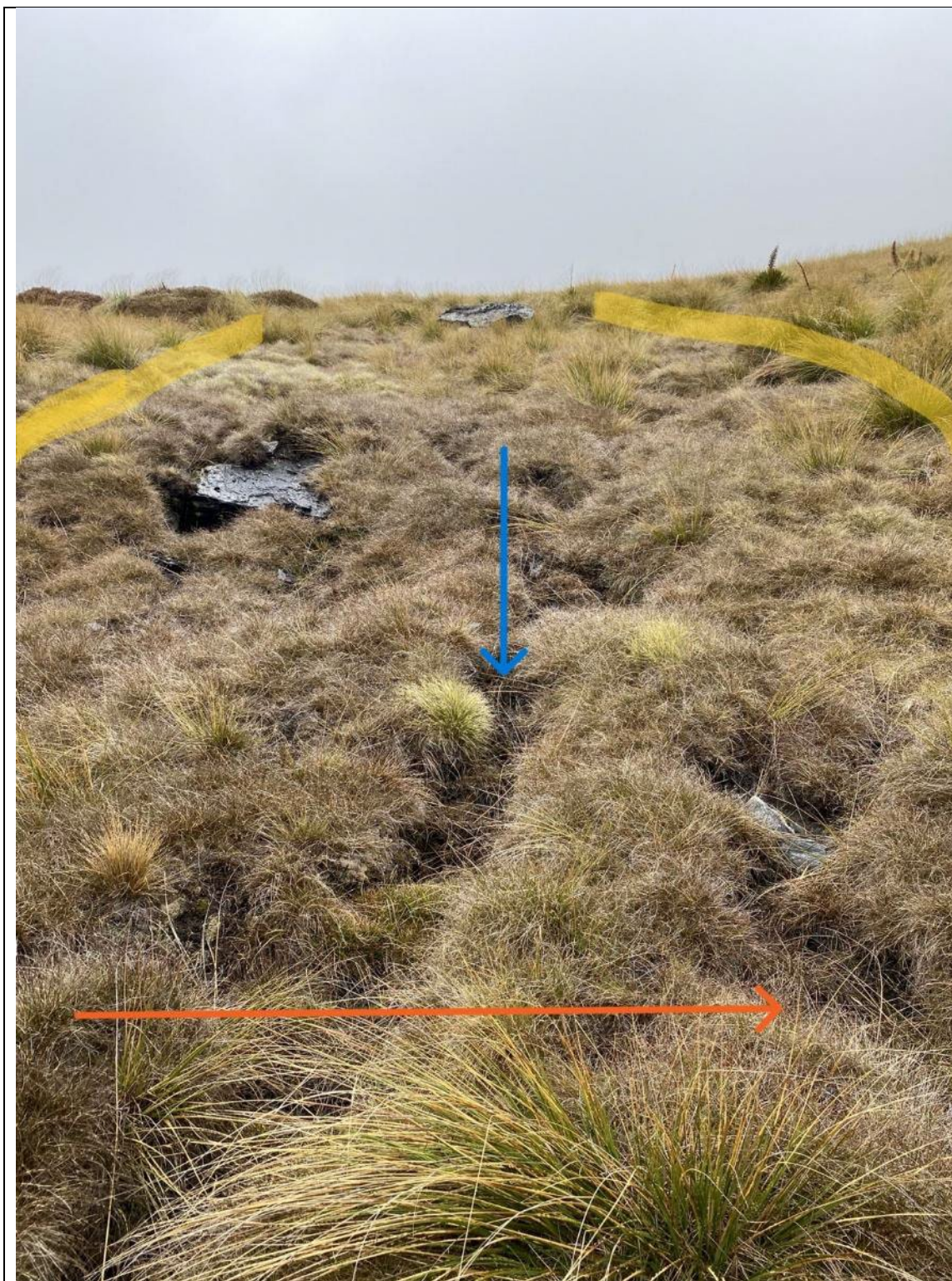
Permeable Track F: No waterway is present, a wetland crossing of approximately 5 m between the yellow lines will be required over the seepage wetland.
