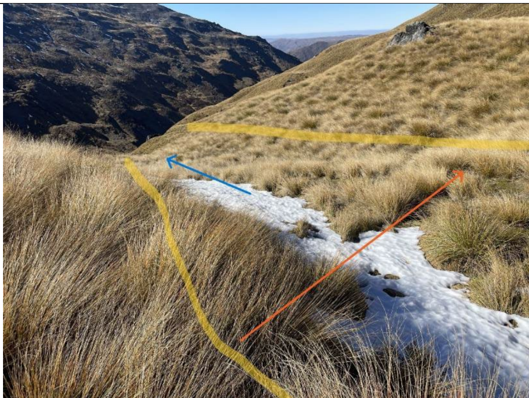
Permeable Track E: No waterway is present, a wetland crossing of approximately 10 m between the yellow lines will be required over the seepage wetland.
