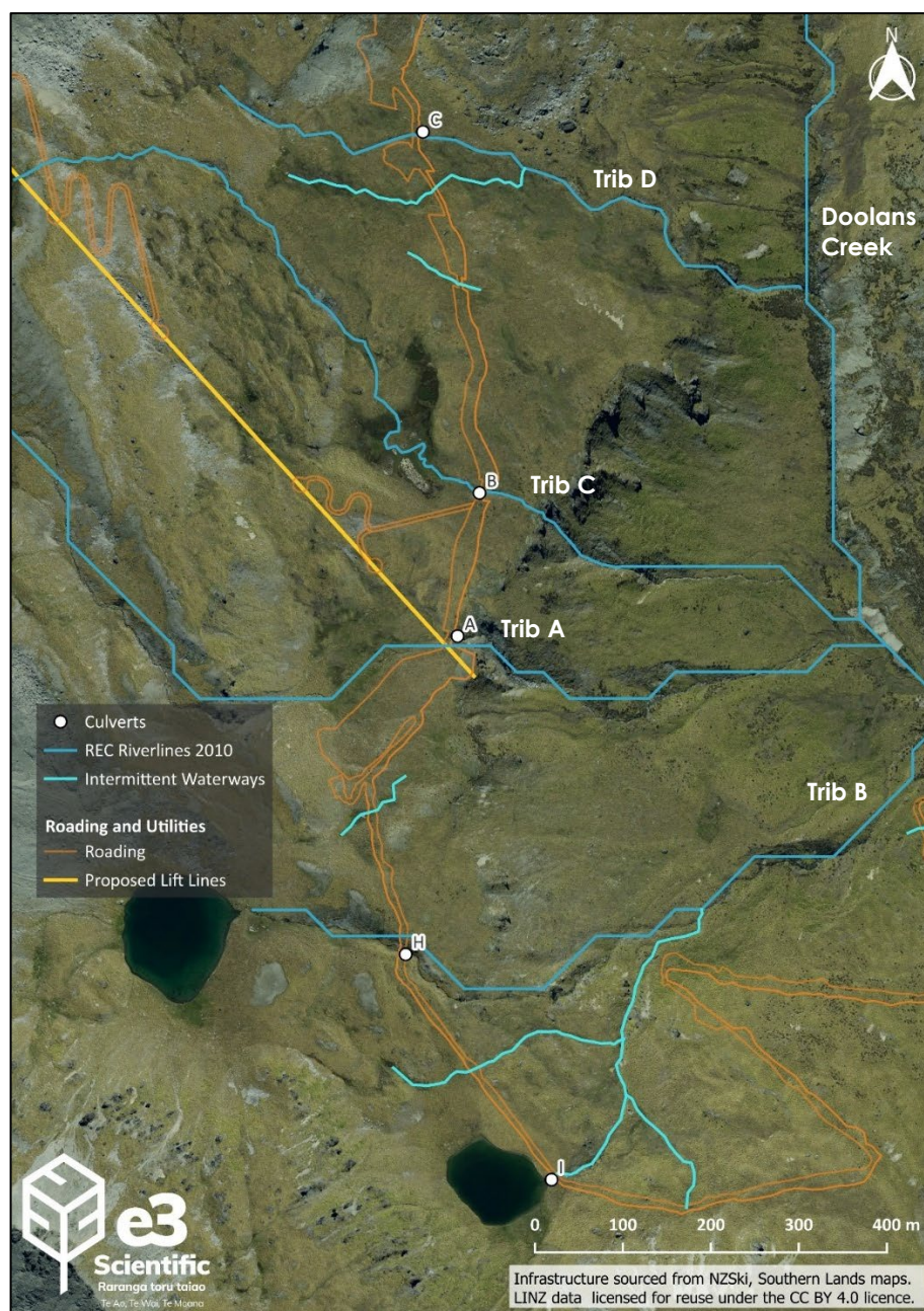
Figure 23: Location of culverts and associated stream habitat loss.
