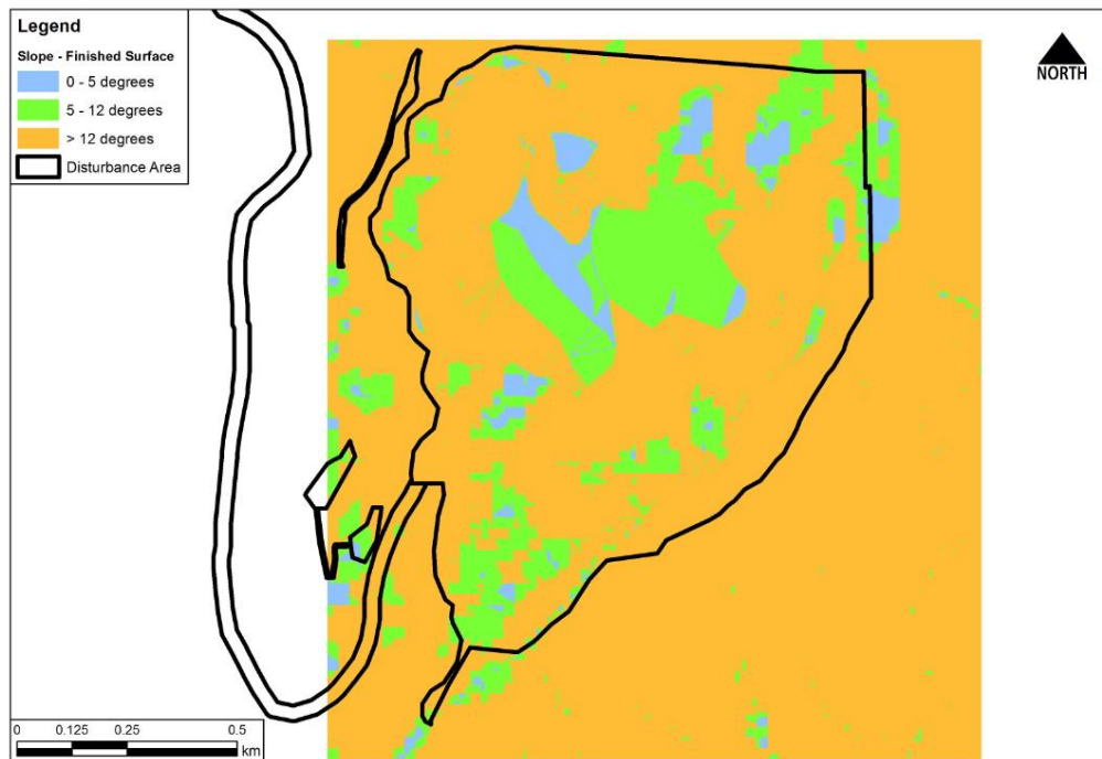
Figure 9. Slope classes of the indicative, finished, rehabilitated surface. This figure uses the same contours as presented in the following Figure 10
