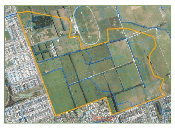
Figure 2: Indicative development catchment area discharging to Old Wairoa Road Catchment, subsidiary of the Pāhurehure Inlet catchment discharging to the Manukau Harbour. Source - Auckland Council GIS
