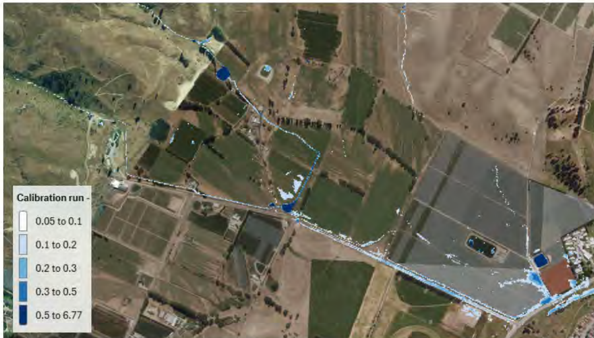
Figure 9 – Tuflow Model Reflecting 23 October Storm Event – Maximum Inundation Depth
