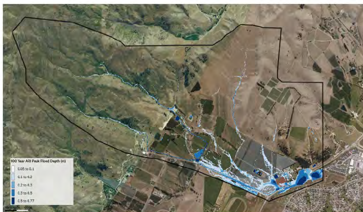
Figure 13 – Current Flooding and Inundation Situation without Stormwater Master planning of the COD site 1% AEP critical durations RCP 8.5 design event
