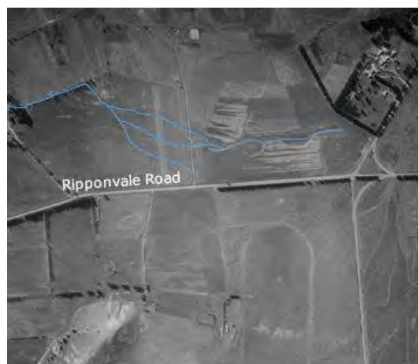
Figure 5B – Retrolens Aerial Image 1950 with visible paleochannels shown in blue
