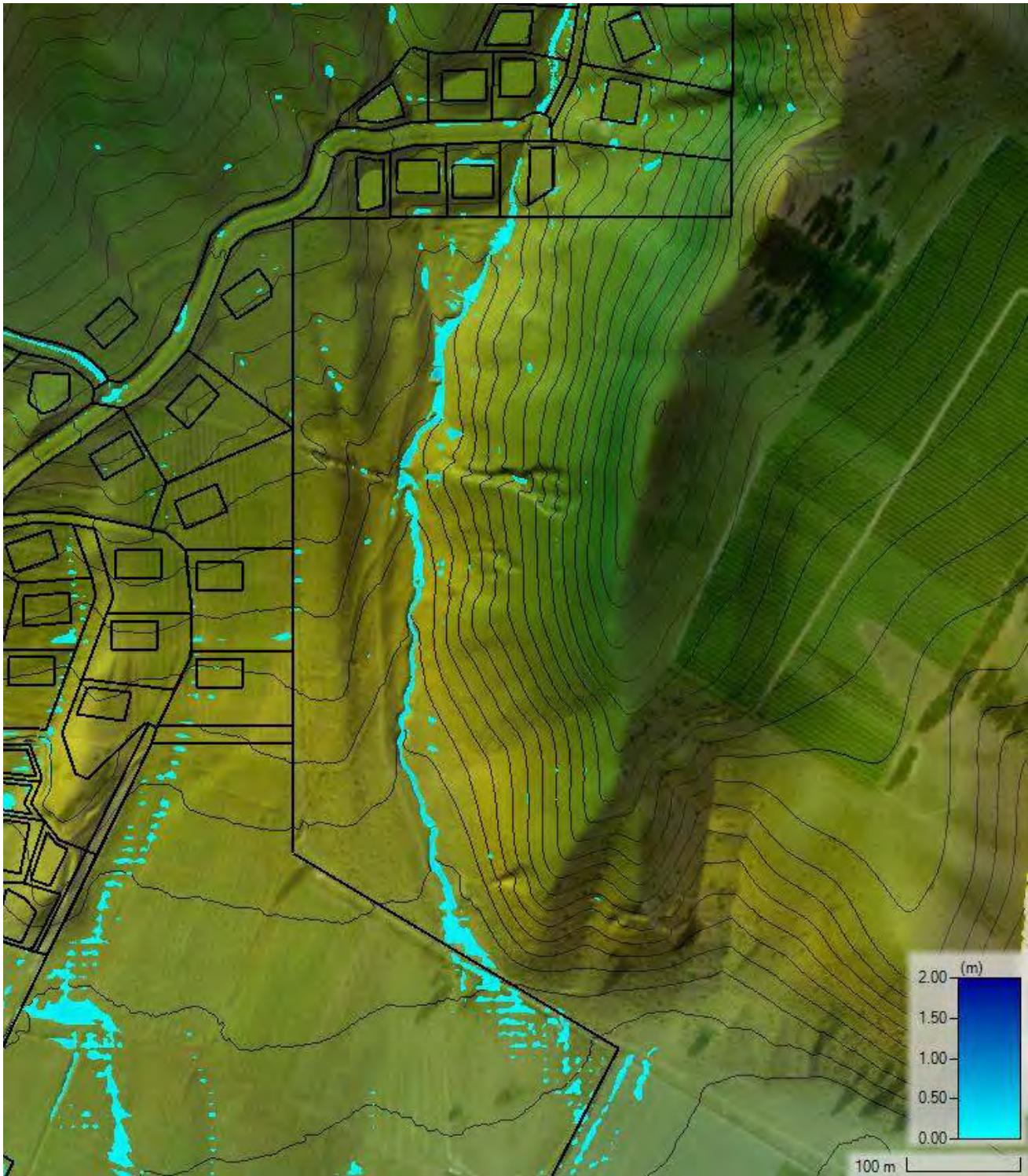
Fig28 – Eastern Catchment – Flooded extents – post dev
