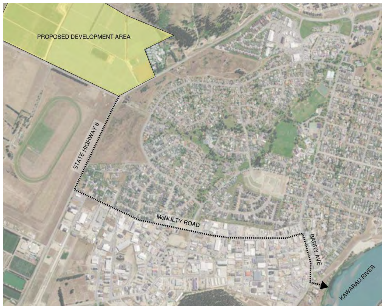
Figure 16 – Overview of stormwater discharge alignment from COD to the Kavarau River
