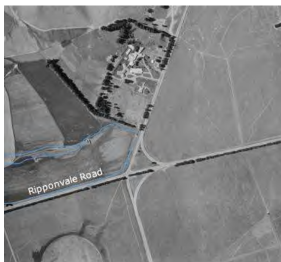
Figure 5C – Retrolens Aerial Image 1962 with visible paleochannels shown in blue
