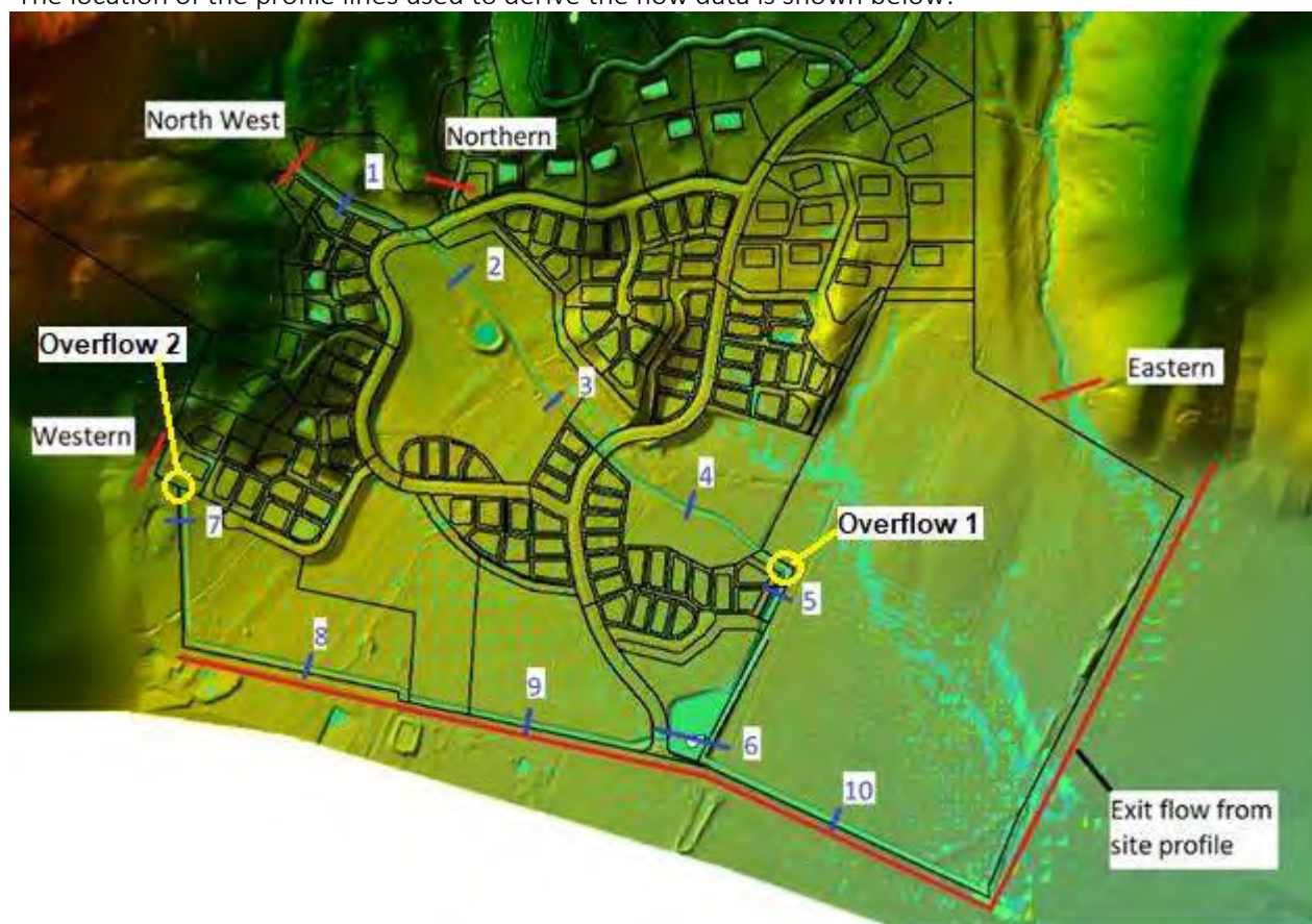
Fig 16 – profile line locations used in analysis. Blue sections indicate channel profile locations. Yellow is the location of channel overflow simulation.
