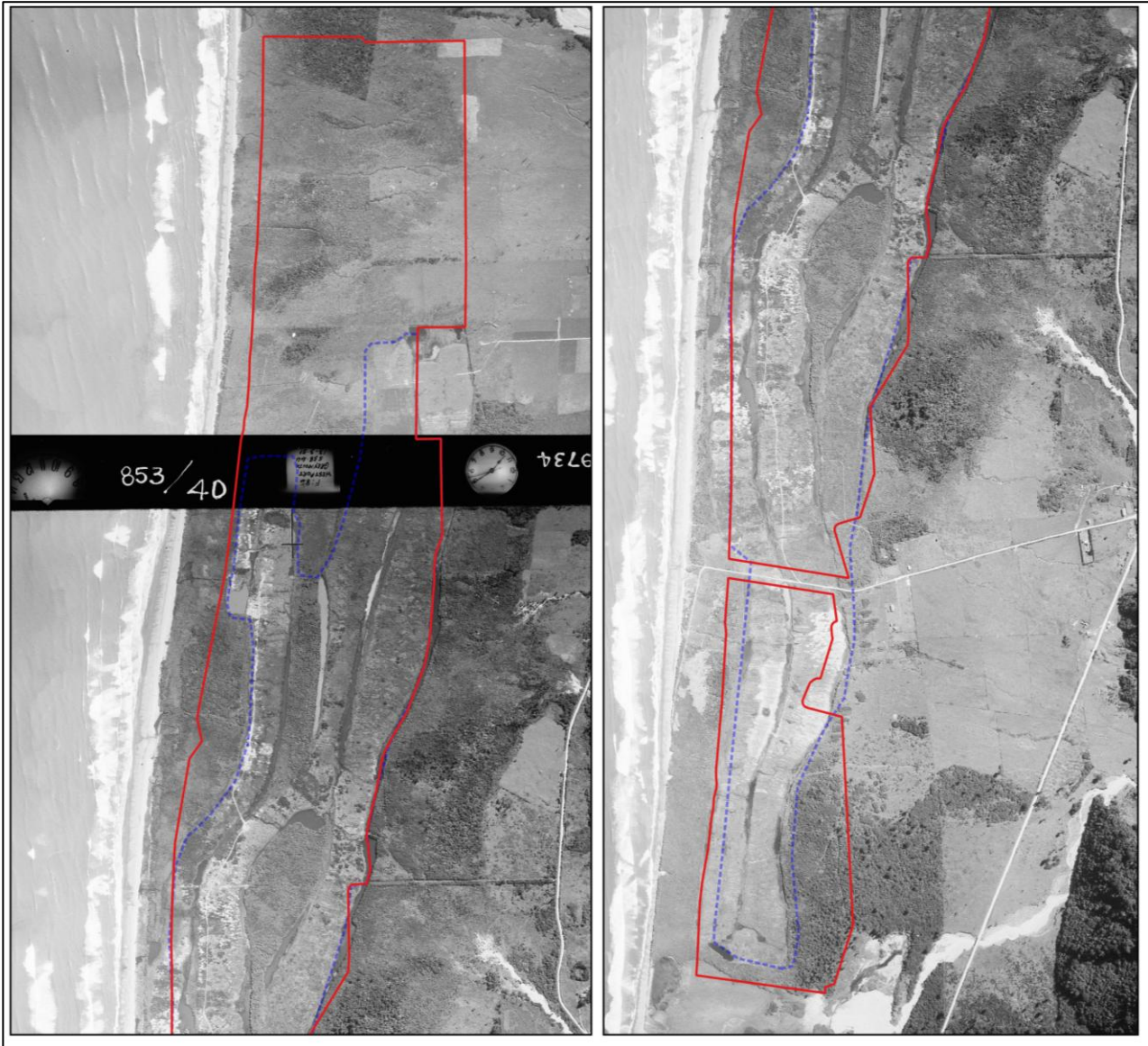
Figure 5-5. Dredged area (blue line) in the project area (red line) in 1951 (Retrolens, 1951).
