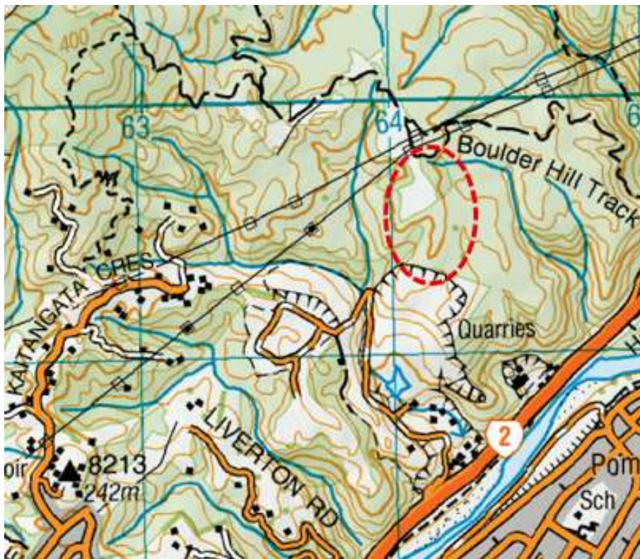
Figure 2.5: Topographic map showing perennial watercourses. Note the generally rolling topography of the proposed OBDA (indicated) and the lack of any streams shown in this area.
