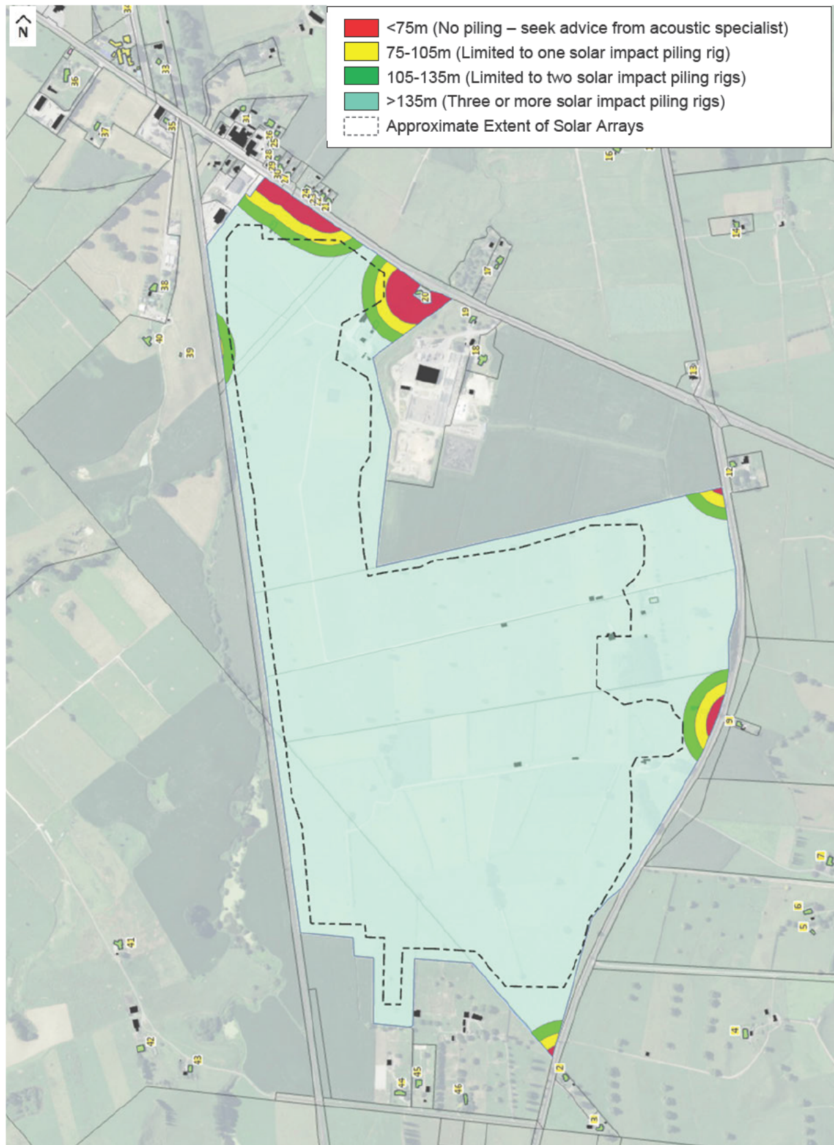
Figure 2 Impact Piling Set Back Distances
