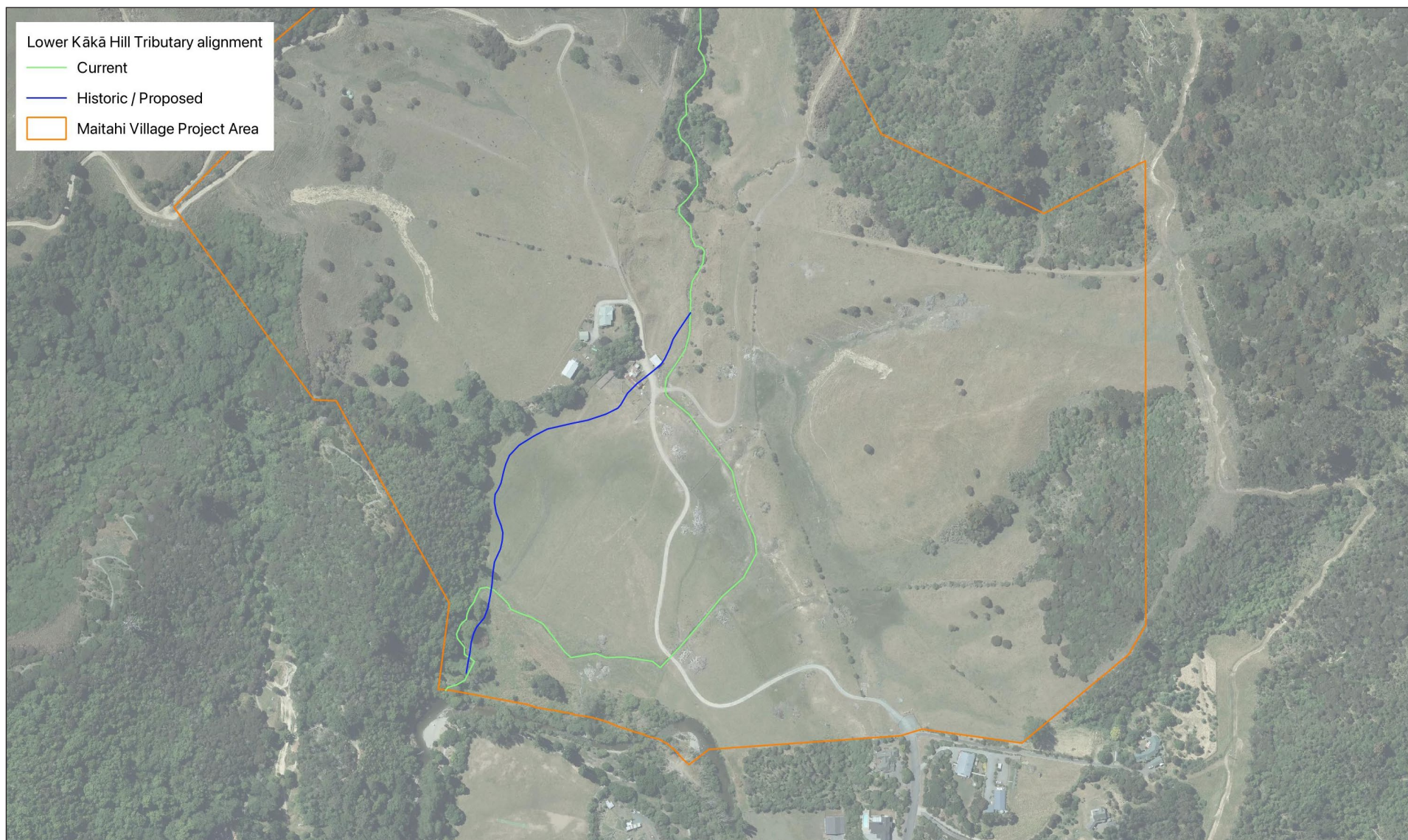
Figure A1. Indicative location of the historic, current and proposed alignments for the Lower Kākā Hill Tributary, within the southern floodplain area. Historic and proposed alignment as per PPC28 Historical & Archaeological Assessment (Attachment B) and the RMM Project Masterplan, respectively.
