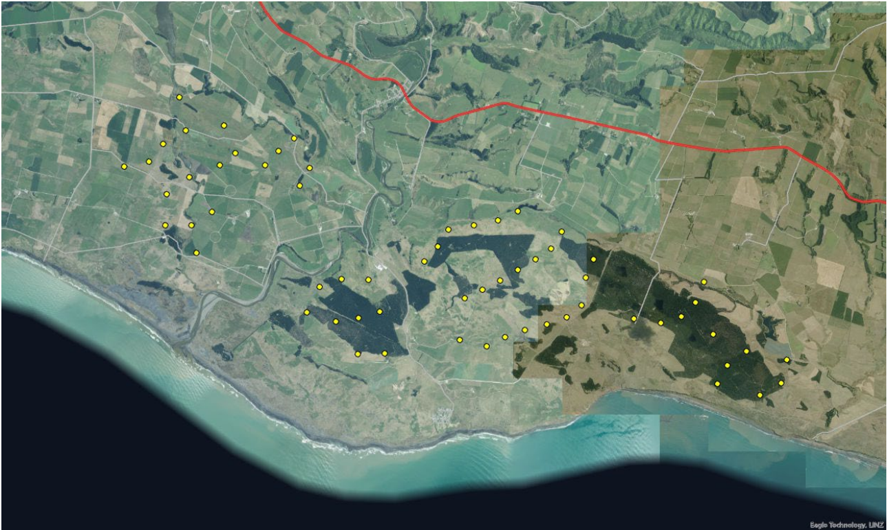
Image 1: Maximum generation capacity indicative layout – 62 turbines
