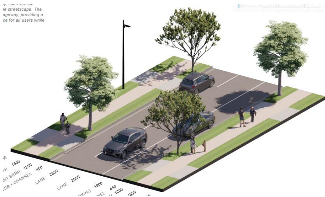
Figure 14: Typical Street Cross Section (Source: Appendix 23)
