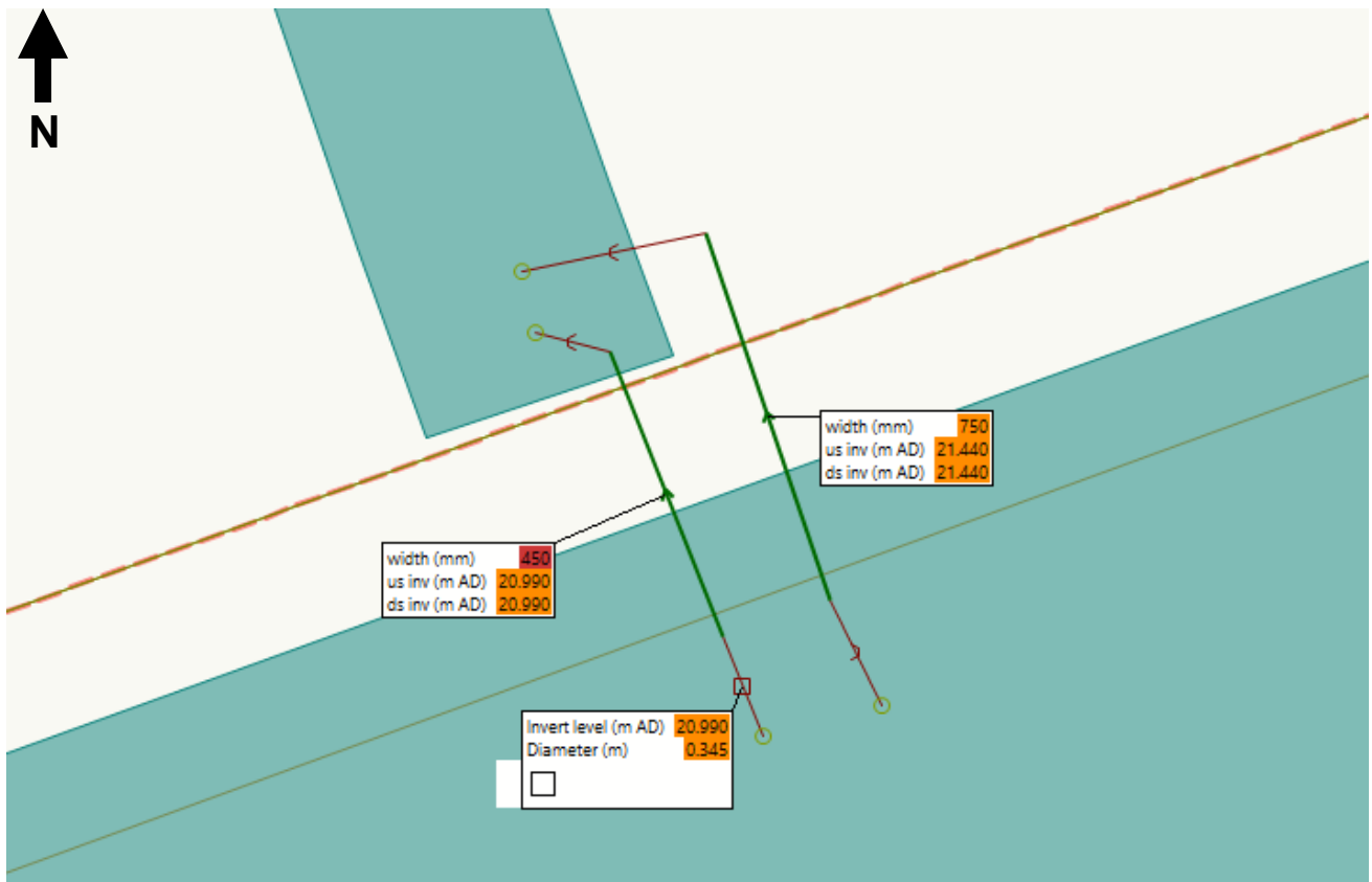
Figure 2-6: Pond 1 outfall pipes configuration in model. Orange flagged values are from Sunfield SWMP (with datum conversion). Red flagged values are inferred/assumed.
