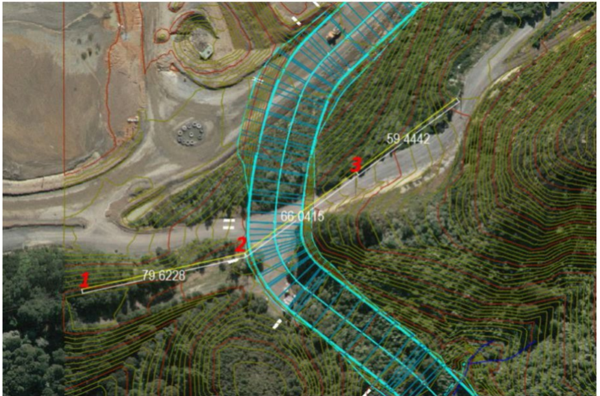
Figure 18: Current Firth powerline location and span distance
