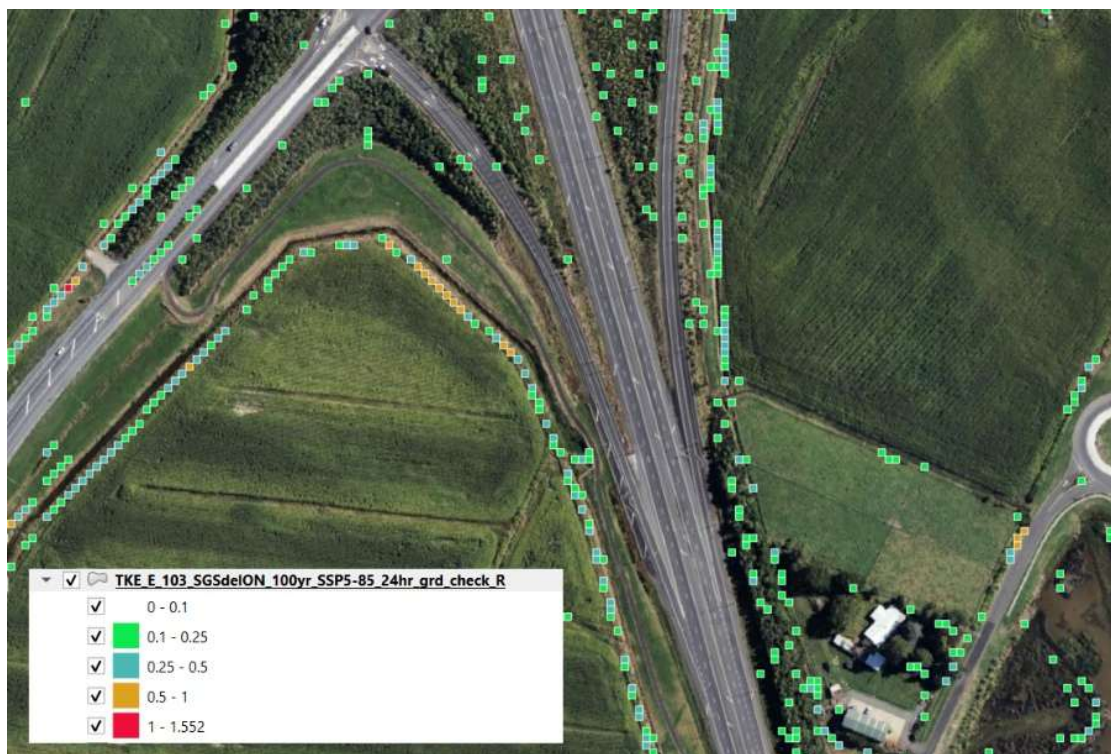
Figure 11. Example of localised SGS cell connectivity identified using the Breakline Detection Delta check (Review Item B2.4).
